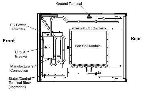
Power and Status/Control wiring must be run in separate conduits or cable trays. Refer to **Appendix D.0 - Installation Drawings** for locations of the various electrical connections between Liebert FS system(s) and UPS system.
